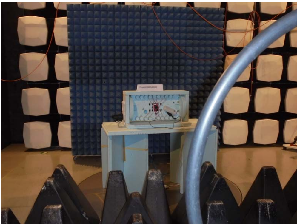
Test setup below 30MHz, long shot view
