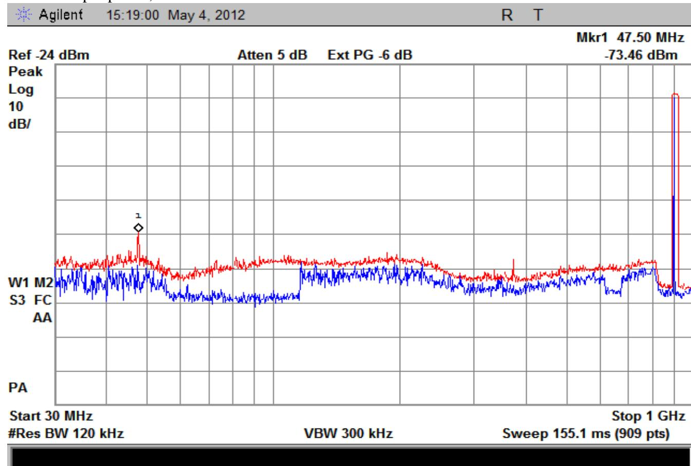
30 dBm output power into external filter Spurious above 1 GHz. 2<sup>nd</sup> harmonic 76 dBm below Fundamental.
