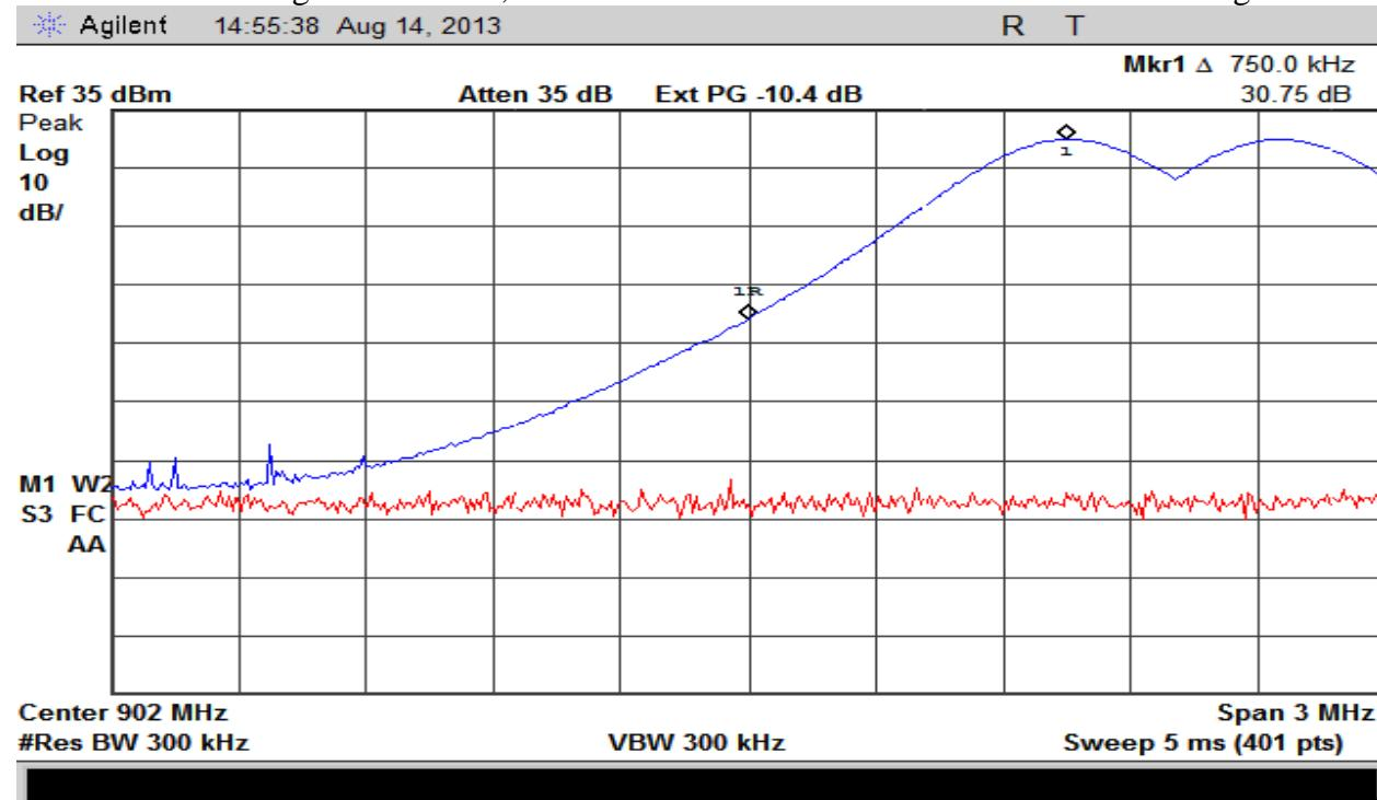
High side.. Band edge is 928 MHz; emissions are more than 20 dB below the inband signal.
