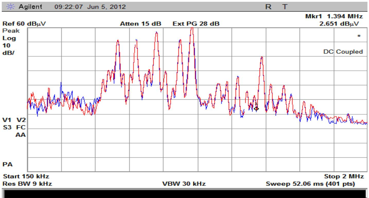
Limit adjusted to 10 meters is 39 dB $\mu$ V in this range. These peaks are ambient emissions.
