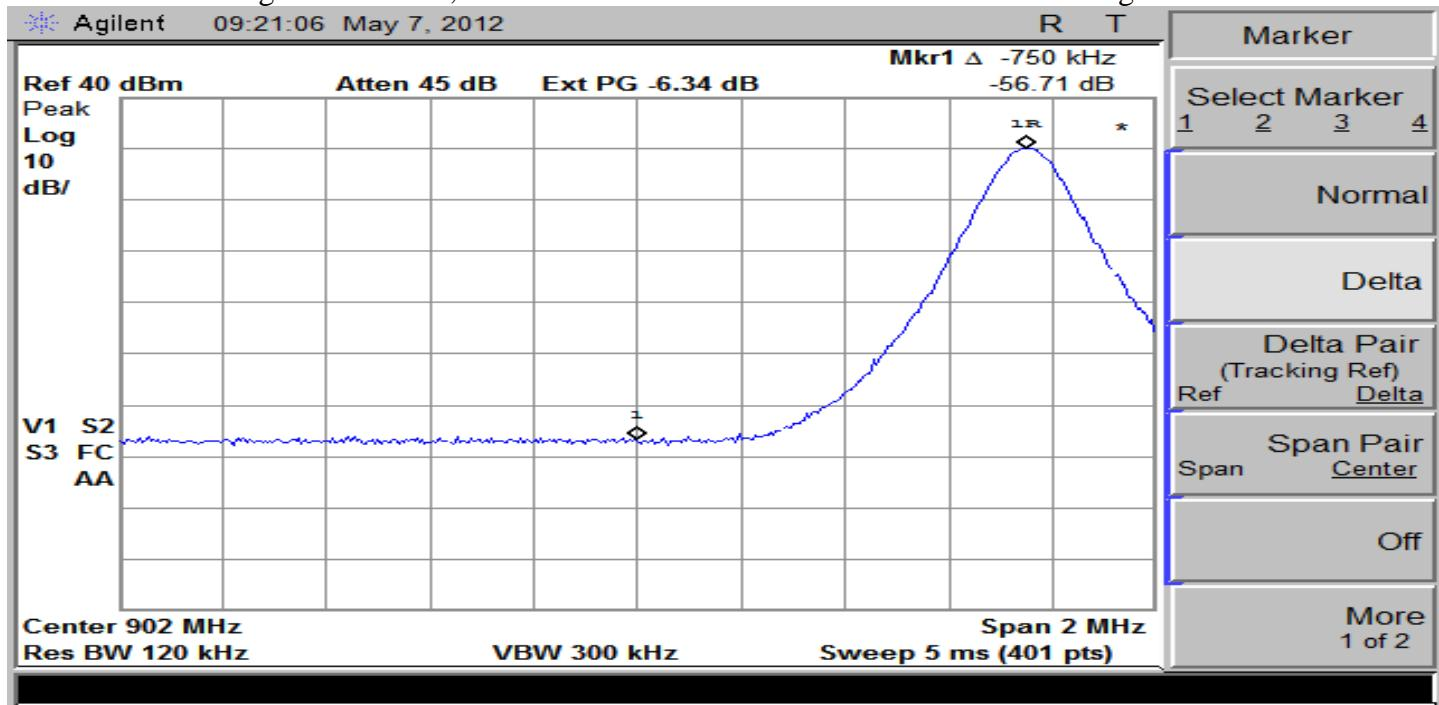
High side.. Band edge is 928 MHz; emissions are more than 30 dB below the inband signal.
