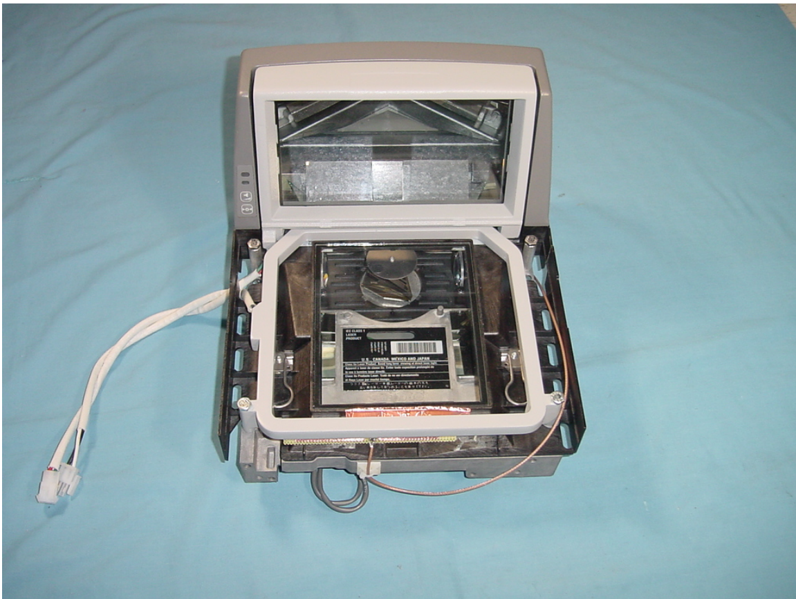
Covers removed from scanner
