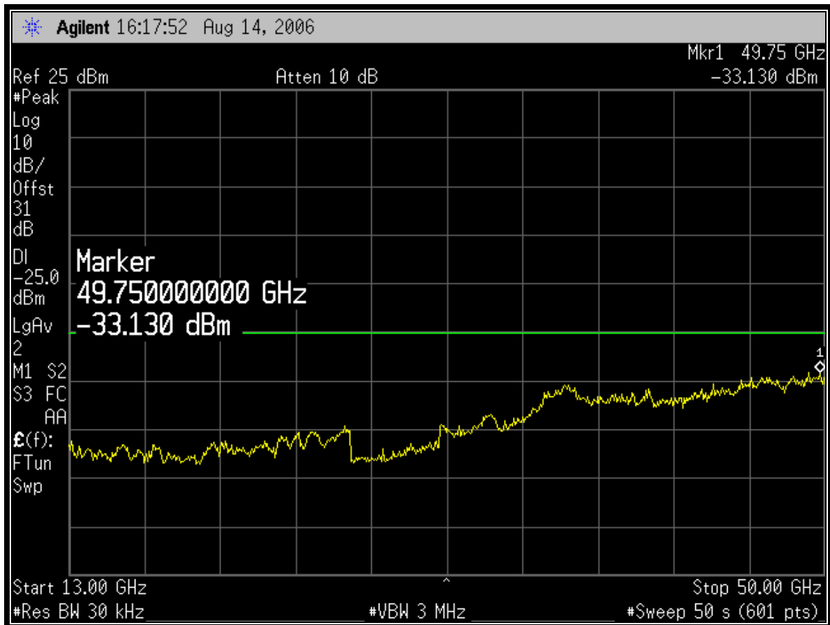
Plot 6-6: Conducted Spurious Emissions; Channel 9 – 4962.5 MHz; 13 GHz – 50 GHz
