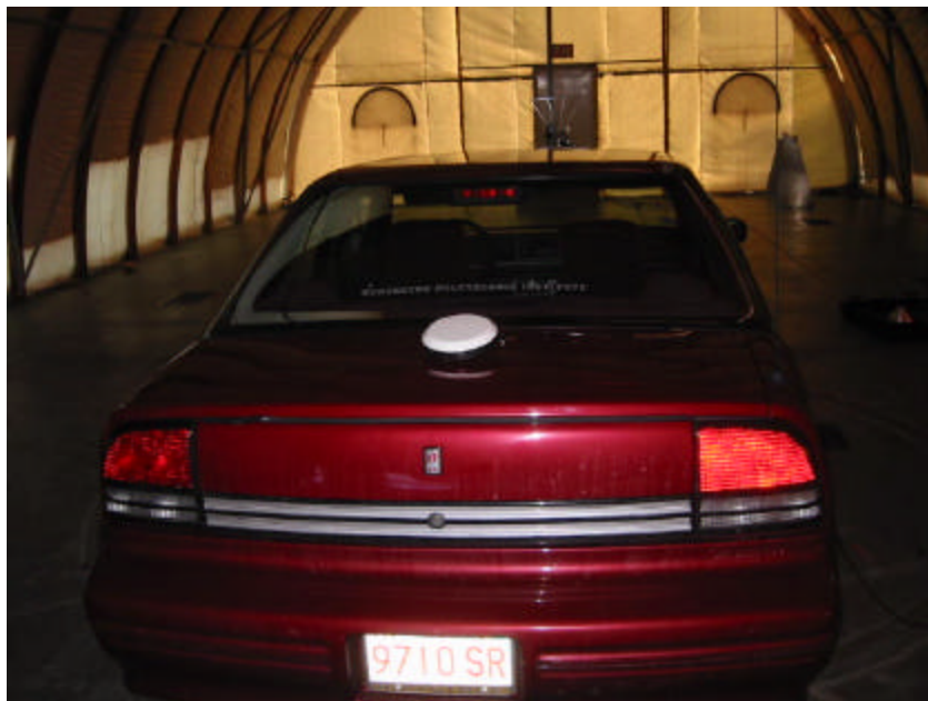
Trunk @ Center Mounting, Puck Antenna
