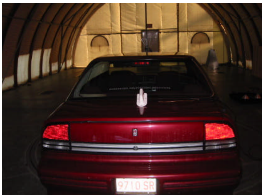
Trunk @ Center Mounting, Transit Antenna
