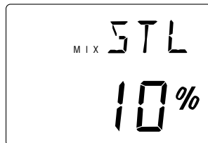
Steering-to-Auxiliary Channel Mixing Adjustment
