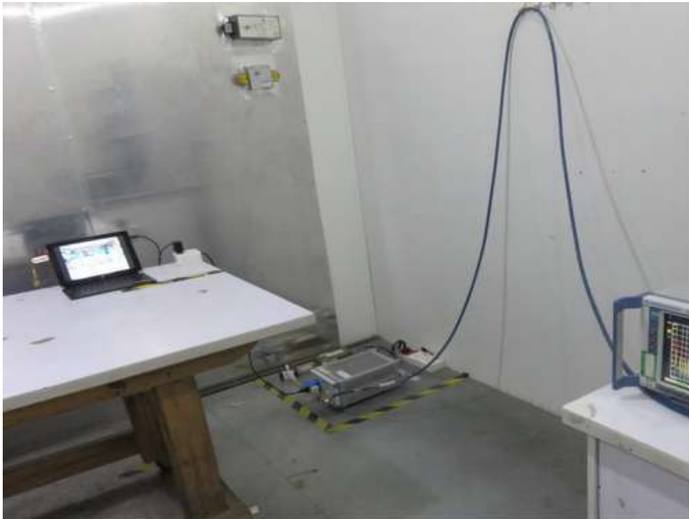
FCC RADIATED EMISSION TEST SETUP
