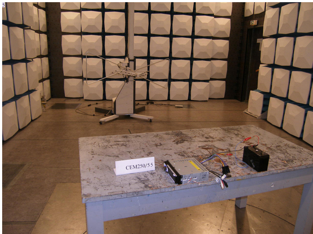
Photograph 1: Set-up for Radiation Measurement below 1GHz
