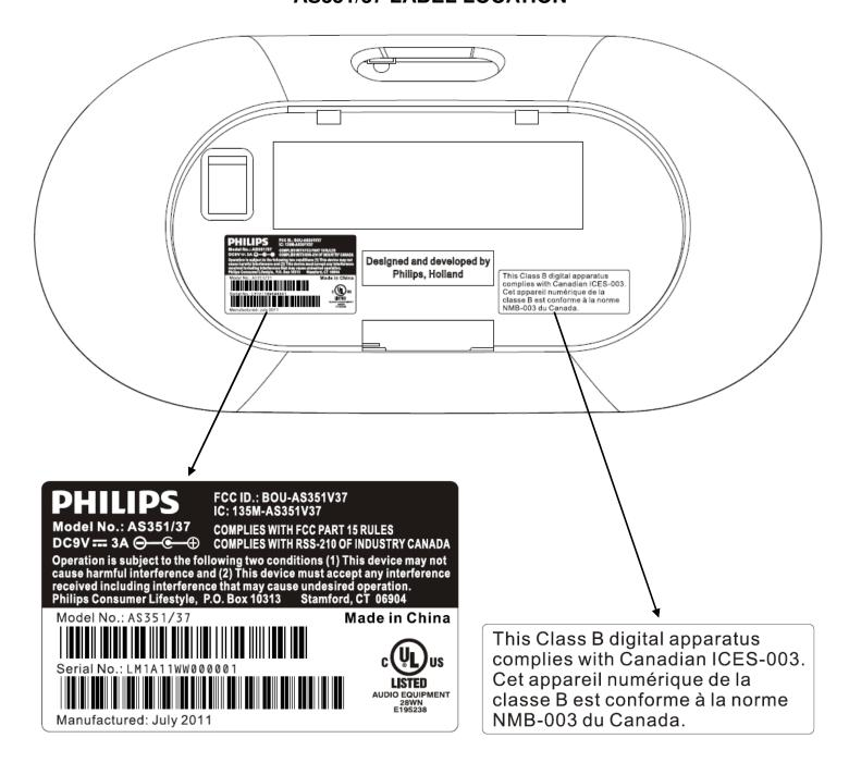
AS351/07 TYPE PLATE LABEL DIM: 45 X 27 mm
