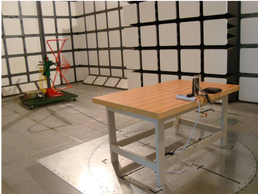
Below 1GHz: Spurious Radiated Emissions - Rear View (powered by adapter)
