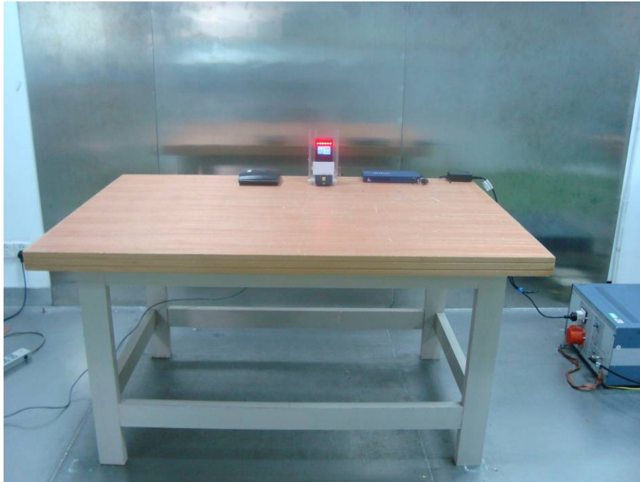
Conducted Emissions - Front View (powered by POE)
