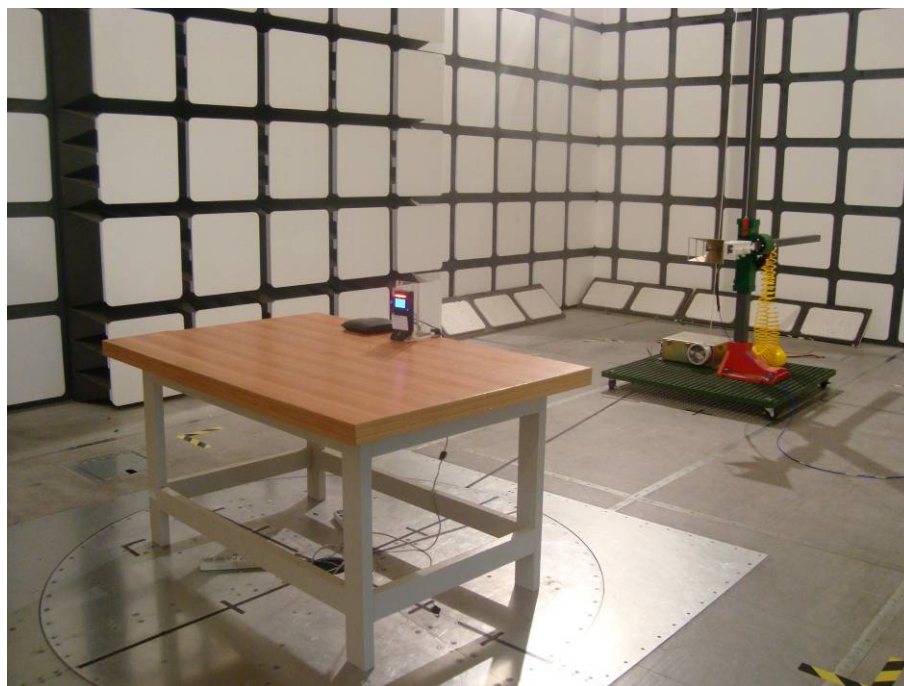
Above 1GHz: Spurious Radiated Emissions - Front View (powered by POE)
