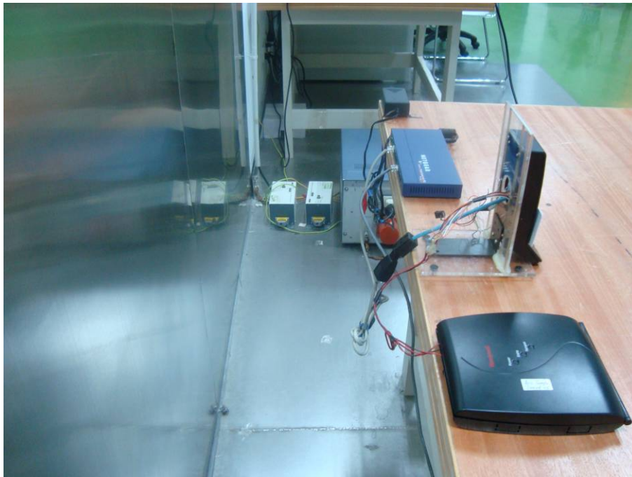
Conducted Emissions - Side View (powered by POE)
