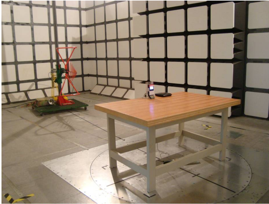
Below 1GHz: Spurious Radiated Emissions - Front View (powered by POE)
