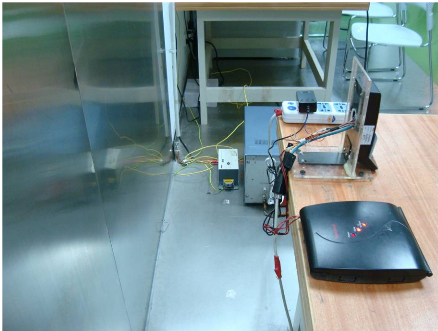
Conducted Emissions - Side View (powered by adapter)
