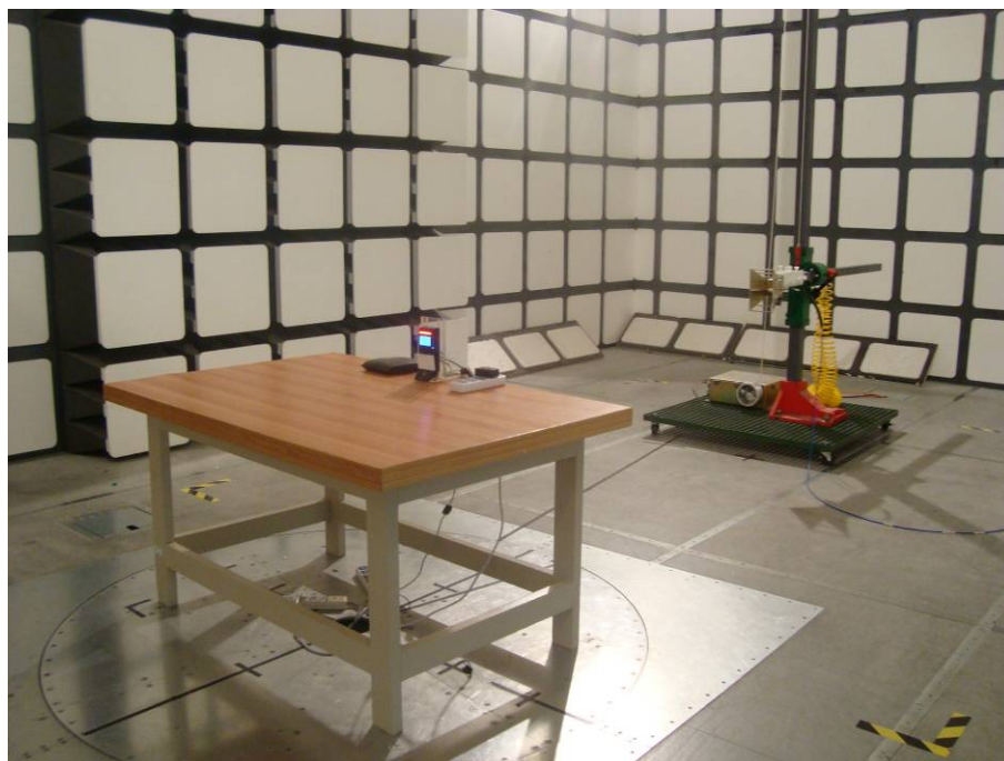
Above 1GHz: Spurious Radiated Emissions - Front View (powered by adapter)
