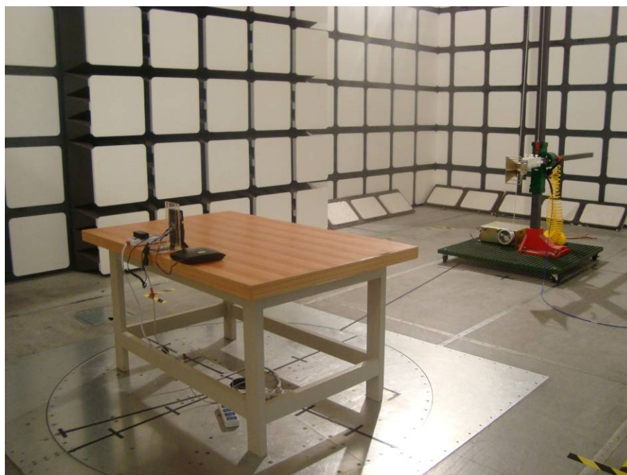
Above 1GHz: Spurious Radiated Emissions - Rear View (powered by adapter)
