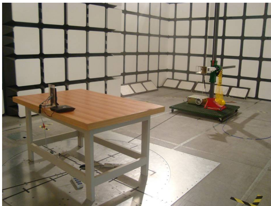
Above 1GHz: Spurious Radiated Emissions - Rear View (powered by POE)
