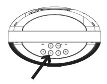
This unit is equipped with a built-in microphone (located below the brand plate on front panel), which allows you to make or end calls of a connected mobile phone through this unit. Make sure your Bluetoothenabled mobile phone is paired with the unit. When there is an incoming call to the connected mobile phone, you will hear an incoming call alert tone from the unit.
