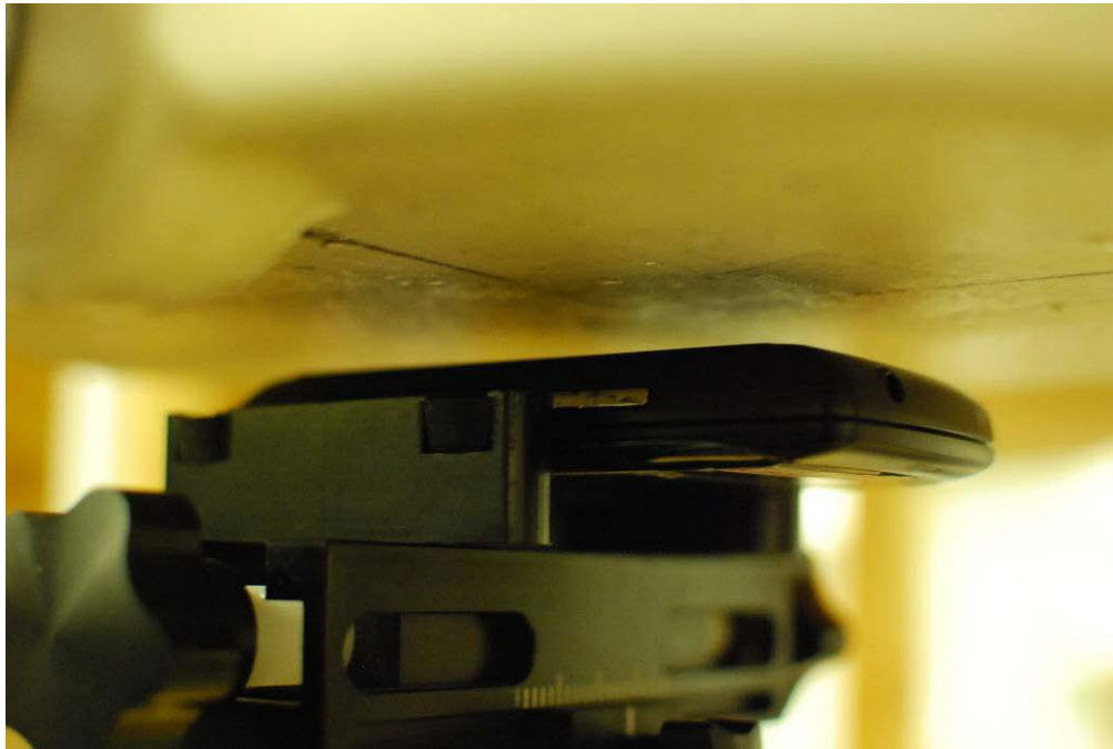
Figure 19-1 SAR Test Setup Photo 1 – Back at 1.0 cm
