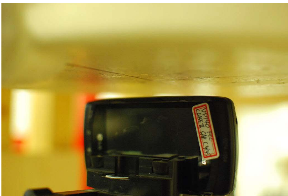
Figure 19-6 SAR Test Setup Photo 6 – Left at 1.0 cm
