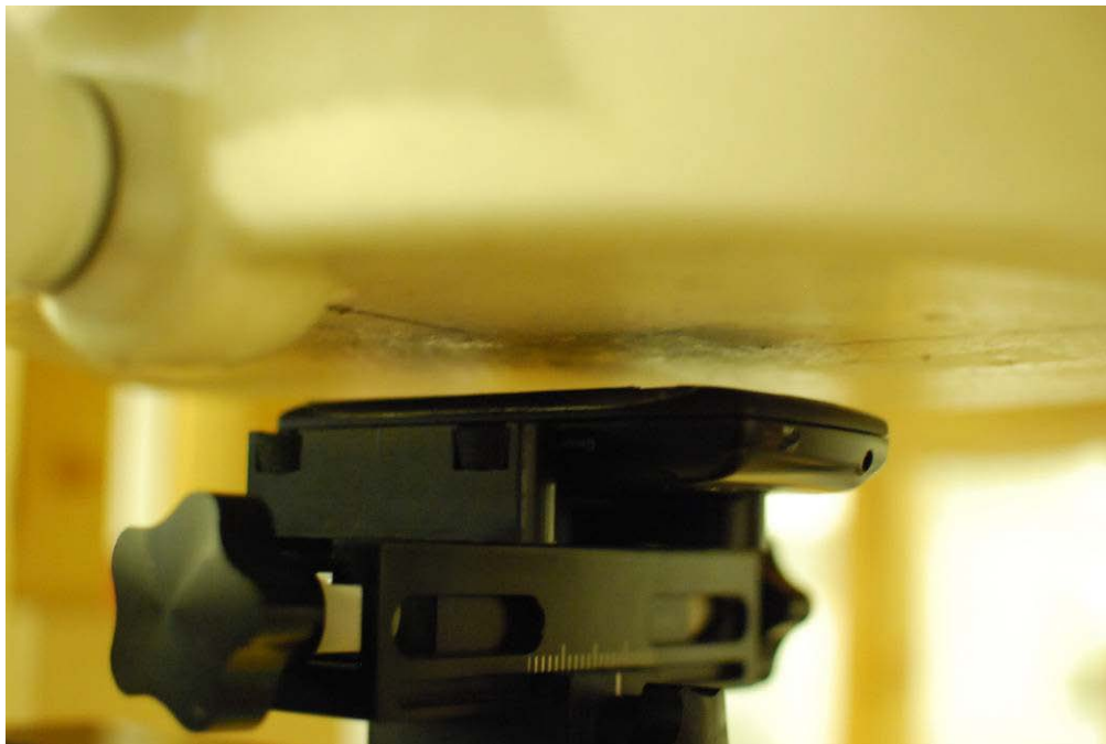
Figure 19-2 SAR Test Setup Photo 2 – Front at 1.0 cm
