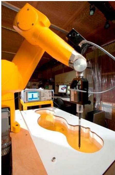
Figure 3-2 SAR Measurement System
