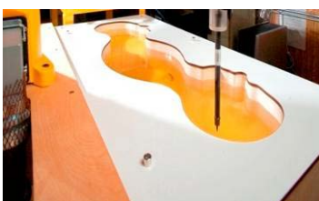
Figure 6-2 SAM Phantom with Simulating Tissue
