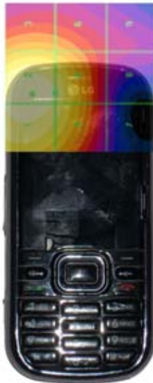
Figure 17-4 E-Field WD Scan overlay
