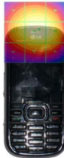
Figure 17-5 H-Field WD Scan overlay
