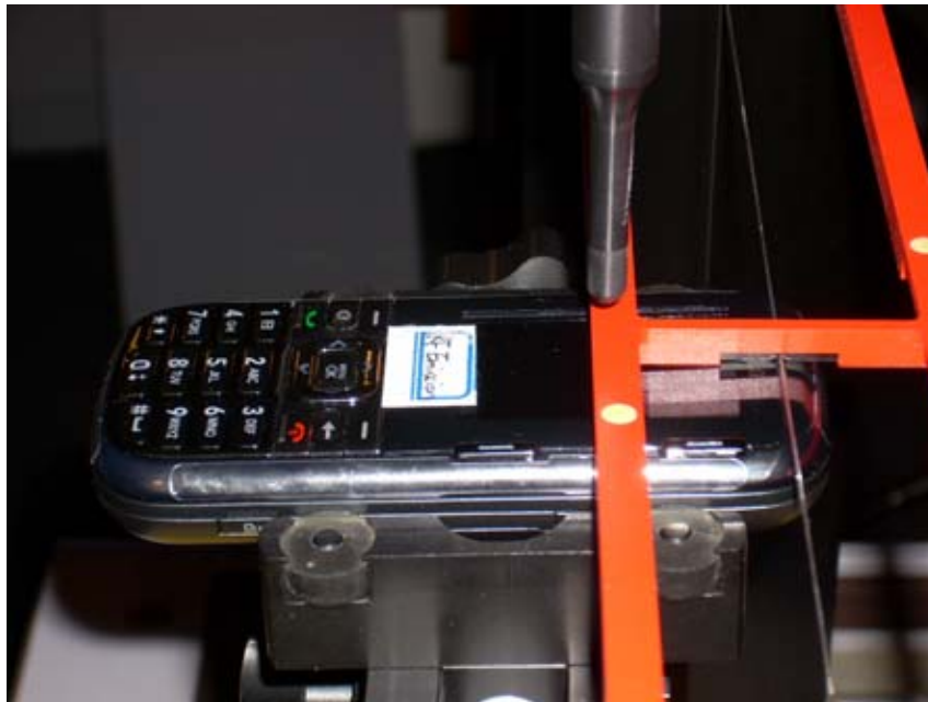
Figure 17-1 Ear Reference Point HAC Phantom Alignment
