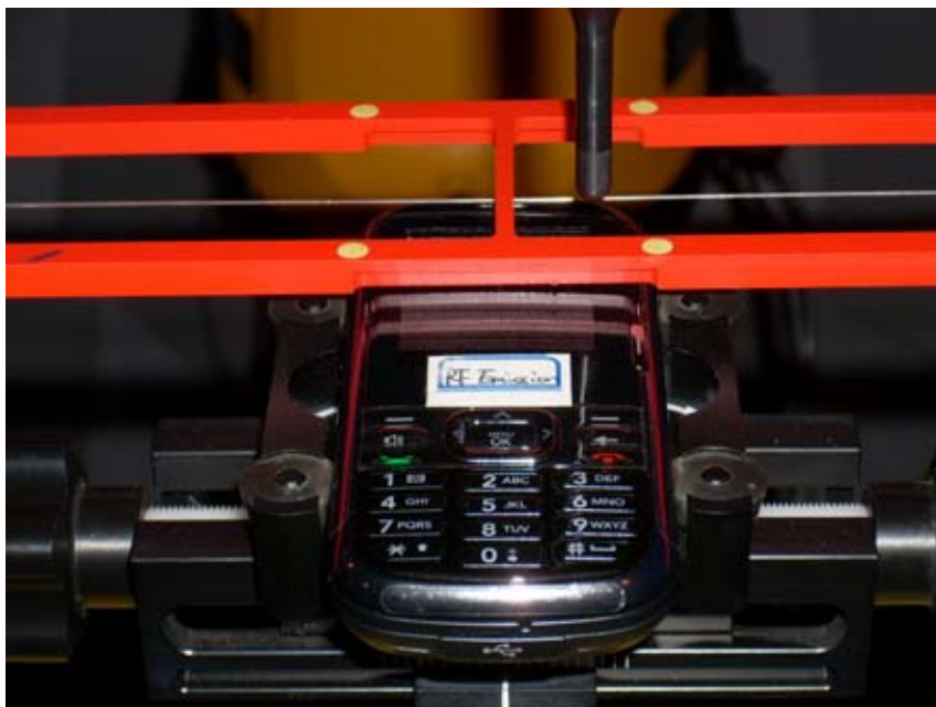
Figure 17-2 HAC Phantom Plane Alignment
