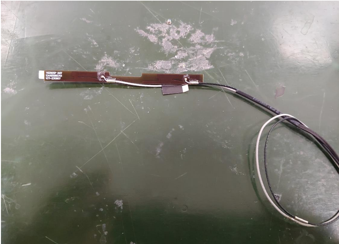
Figure 45 L1LRF015-CS-H, WLAN Combo Antenna
