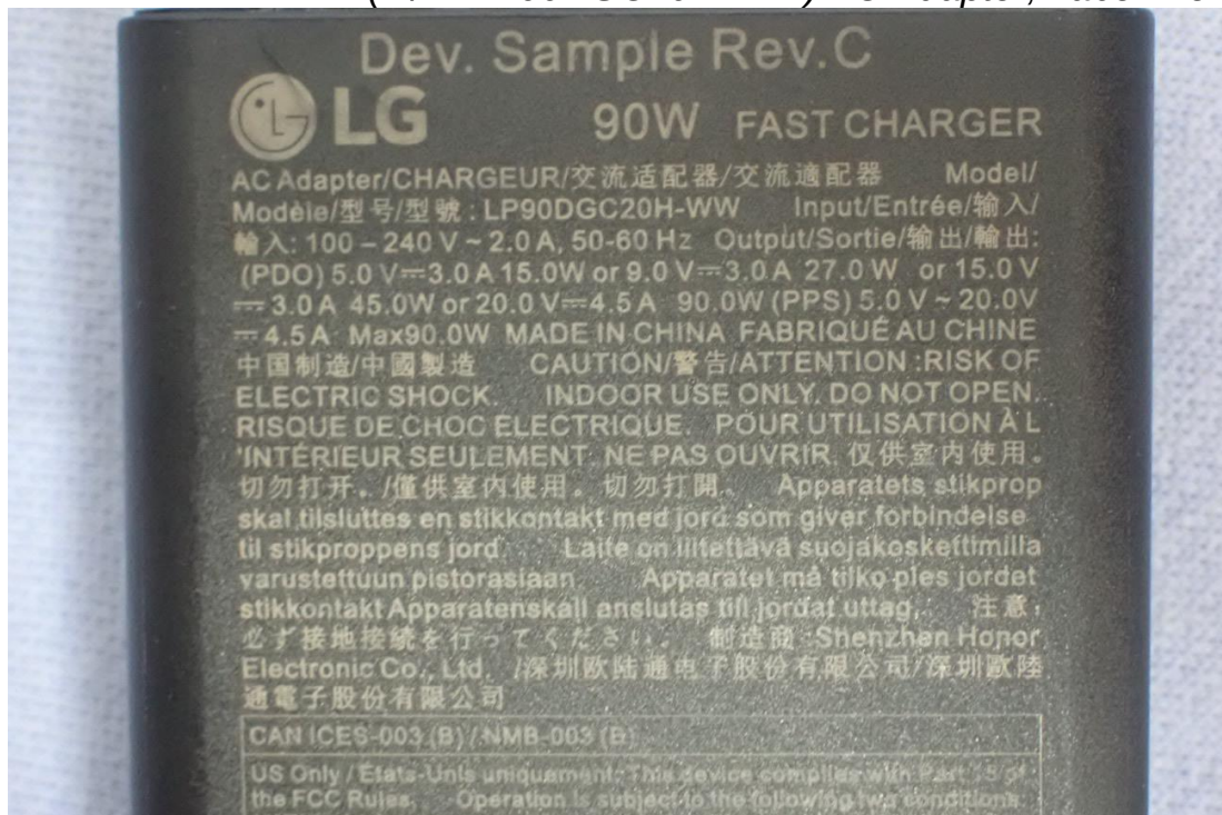
Figure 71 (M/N: LP90DGC20H-WW) AC Adapter, Label View
