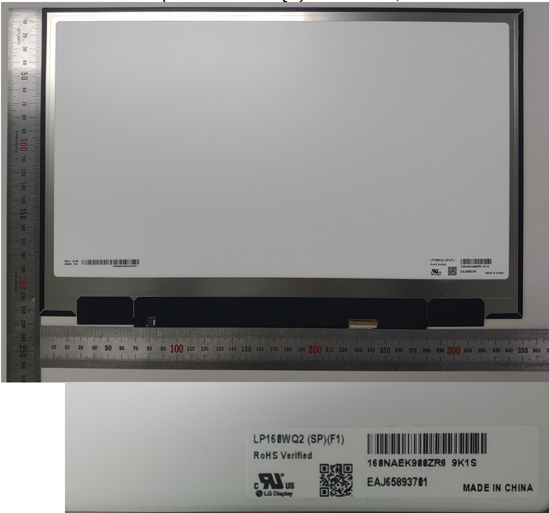
Figure 42 (M/N: LP160WQ2) LCD Panel, Back & Label View
