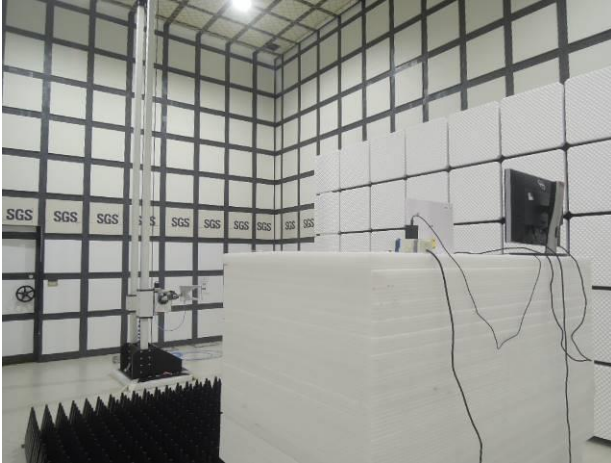
FCC 15_247 WLAN Radiated Setup
