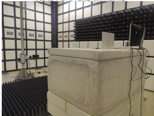
FCC 15_407 WLAN 6E Radiated Setup
