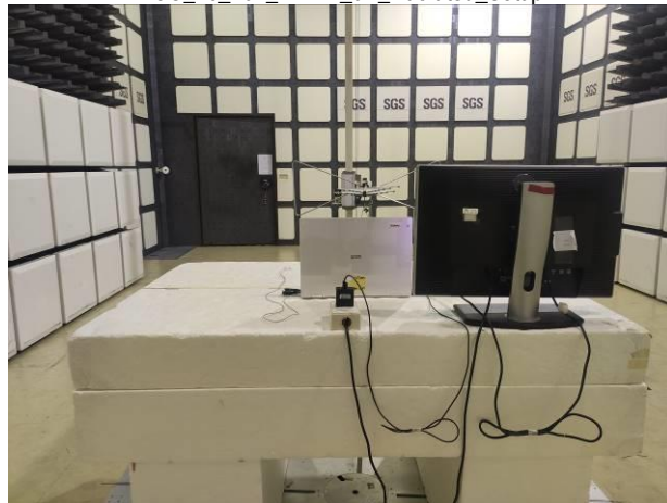
FCC 15_407 WLAN 6E Radiated Setup
