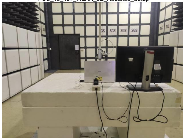
FCC 15_407 WLAN 6E Radiated Setup
