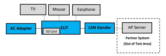
3.9.2. EUT Configuration for RF Conducted Test Items
