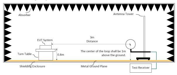
6.1.3. Setup Diagram for 30-1000MHz
