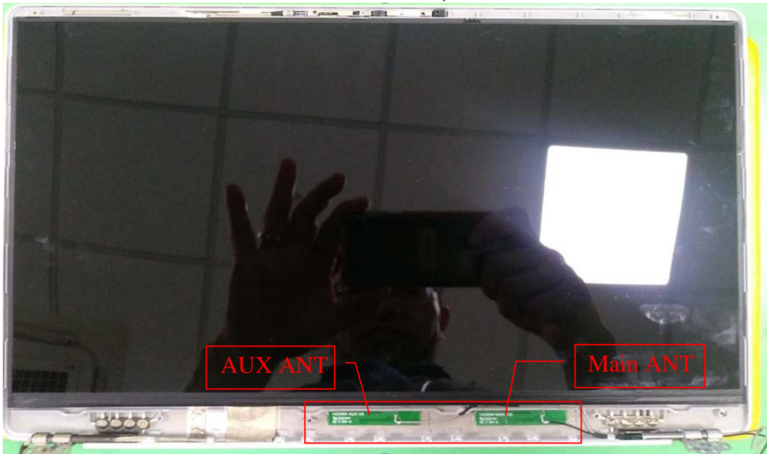
Figure 32 M/N WA-P-LBLB-04-069, WLAN Combo Antenna Position
