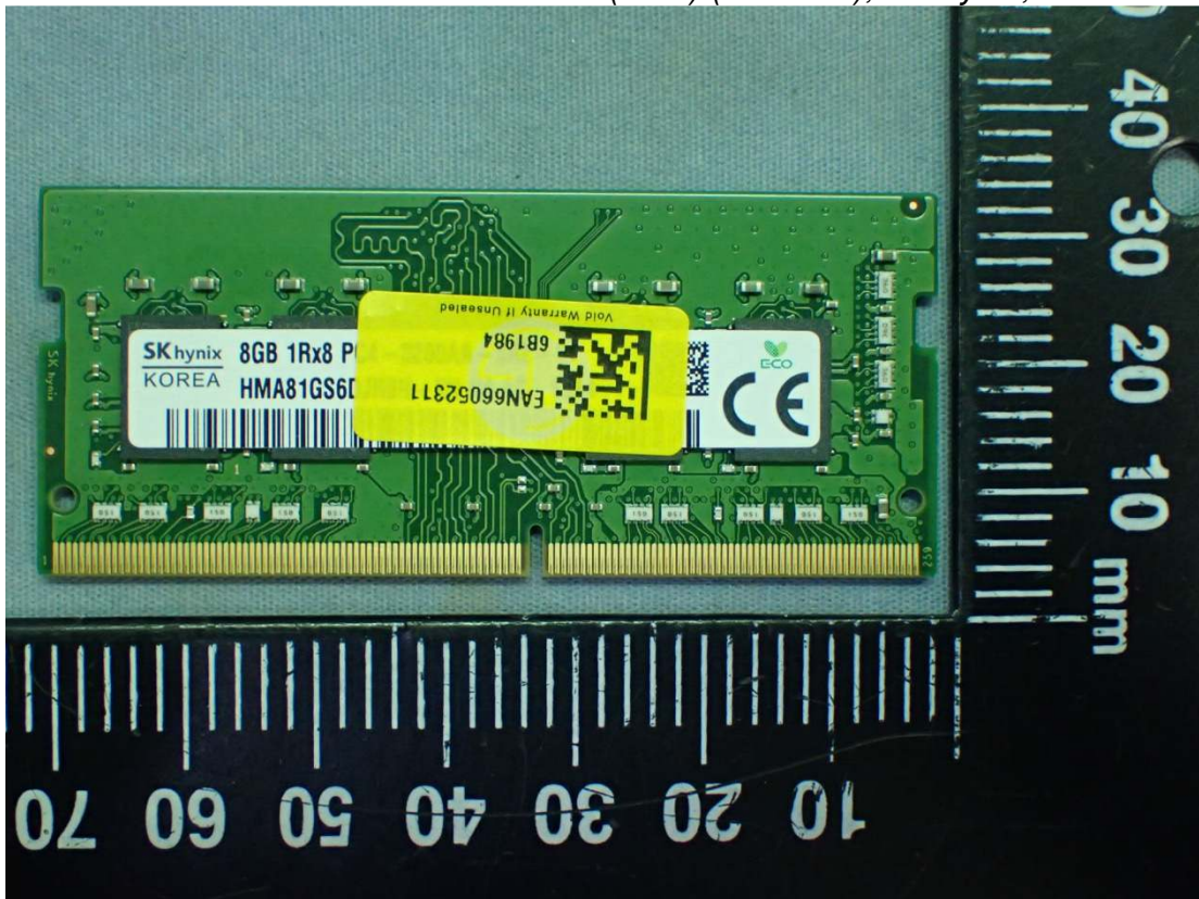
Figure 45 RAM (8GB) (On Card), SK hynix, Front View
