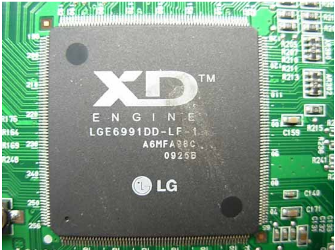
FIGURE 4 LCD MONITOR (M/N: LSM1850HU) CHIP ON MAIN BOARD
