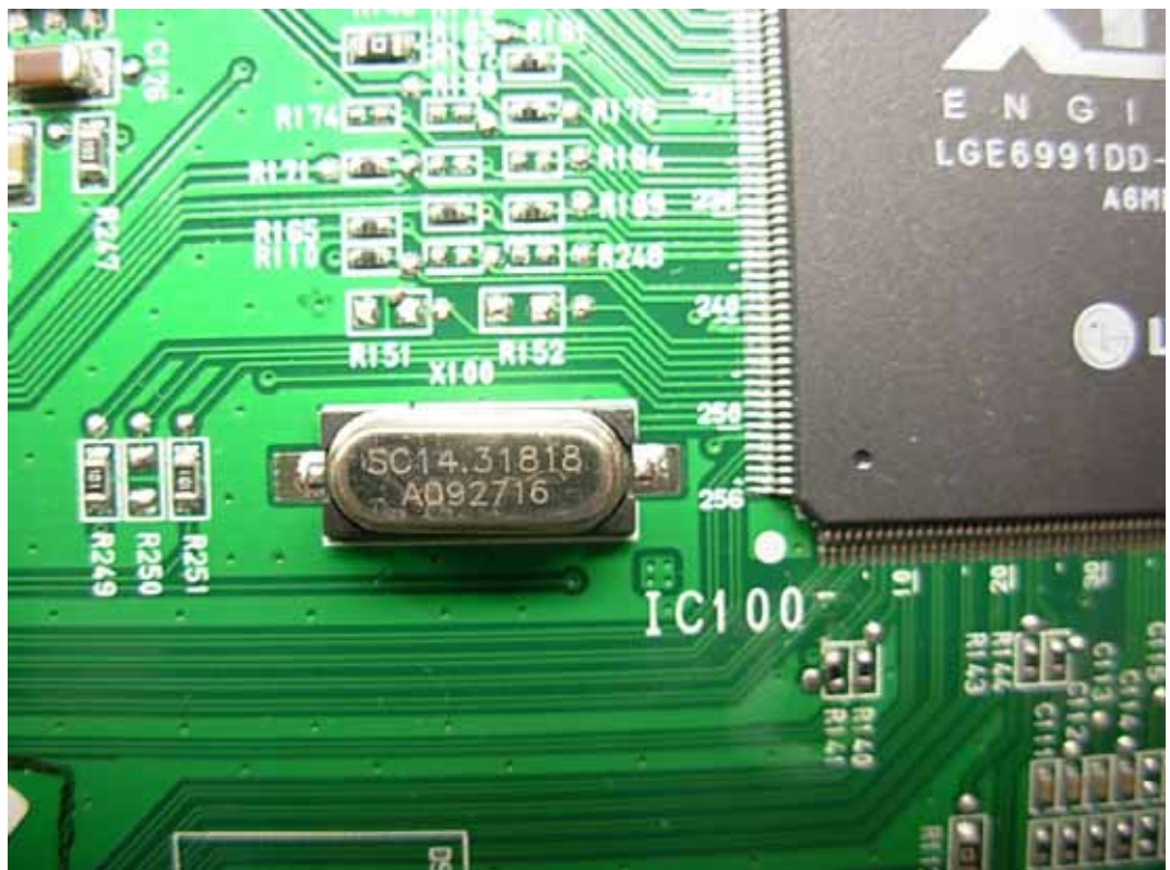
FIGURE 5 LCD MONITOR (M/N: LSM1850HU) CRYSTAL ON MAIN BOARD
