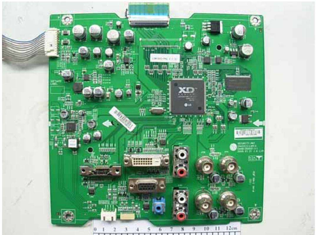
FIGURE 2 LCD MONITOR (M/N: LSM1850HU) MAIN BOARD (COMPONENT SIDE)
