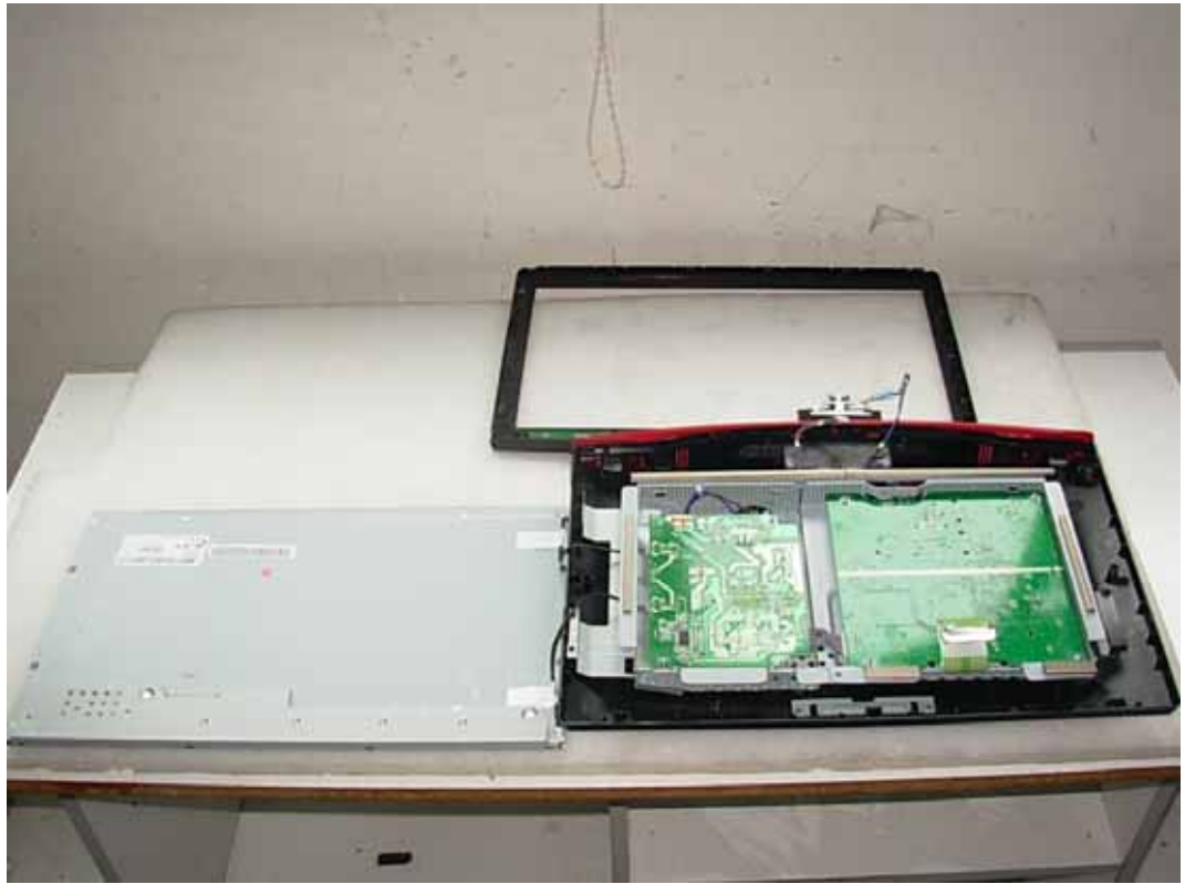
FIGURE 1 LCD MONITOR (M/N: LSM1850HU) COVER REMOVED
