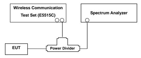
(Configuration of conducted Emission measurement) Test Procedure
