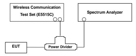
(Configuration of conducted Emission measurement)
