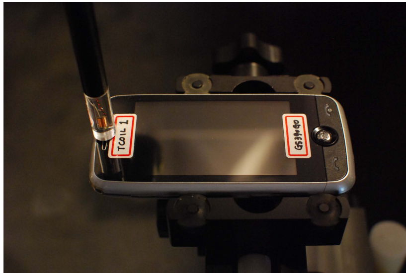
Figure 12-2 Test Setup for Wireless Device
