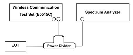
(Configuration of conducted Emission measurement) Test Procedure
