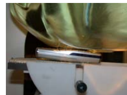
Figure A.3 Left Head SAR Test Setup -- Cheek / Touch Position --
