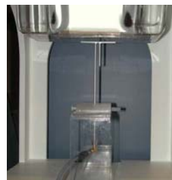
Figure A.0 Dipole Validation Test Setup
