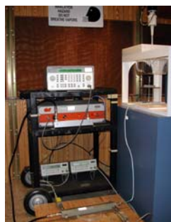
Figure A.0 Dipole Validation Test Setup
