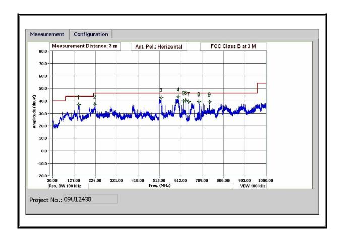
Note: Measurements in this frequency range are made simultaneously on control box (Support Equipment) and Television (Host).
