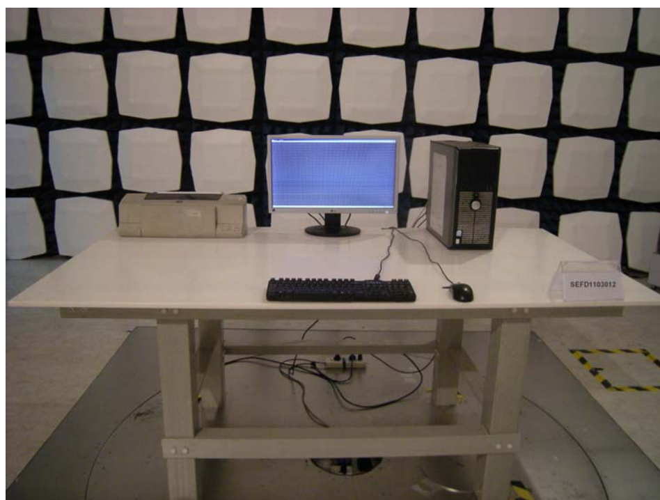
Front View of Radiated Emission Test
