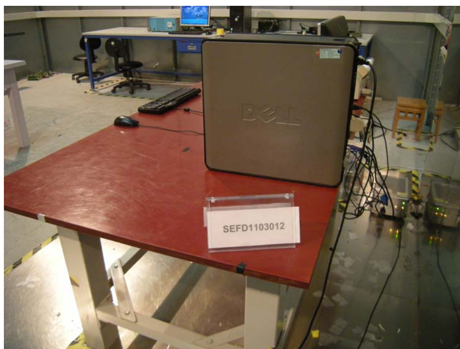
Back View of Conducted Emission Test
