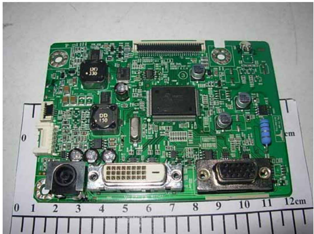
FIGURE 2 LCD MONITOR (M/N: E2050TV) MAIN BOARD (COMPONENT SIDE)
