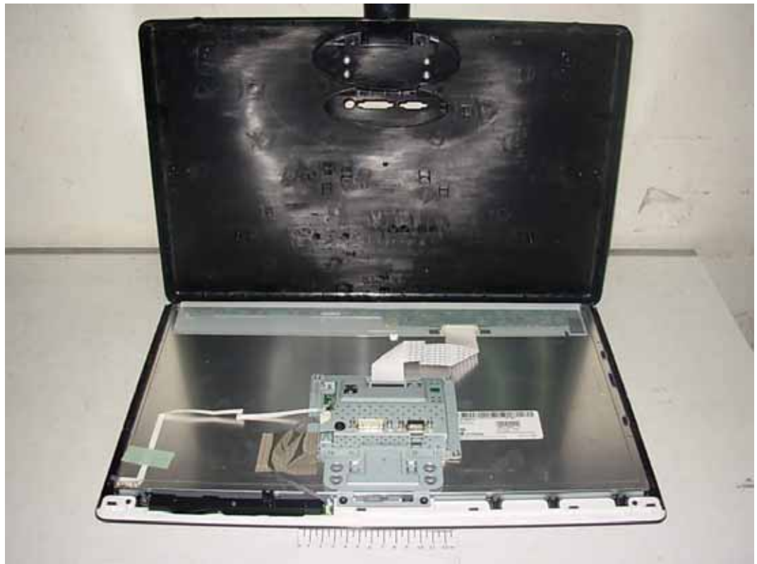
FIGURE 1 LCD MONITOR (M/N: E2050TV) COVER REMOVED
