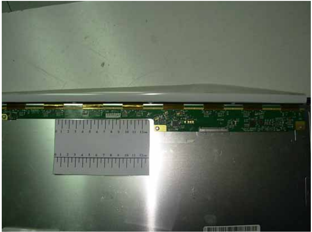
FIGURE 9 LCD MONITOR (M/N: E2050TV) LCD PANEL MAIN BOARD (COMPONENT SIDE)
