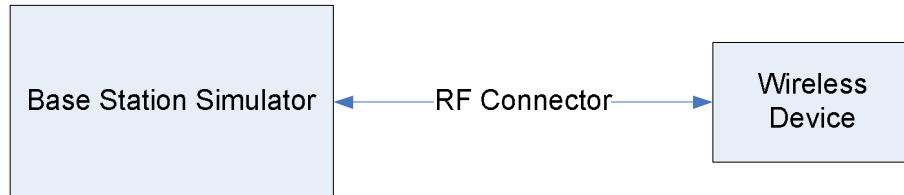
Figure 9-1 Power Measurement Setup
