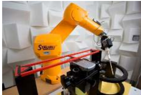
Figure 5-5 SPEAG Robotic System
