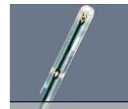
Figure 5-2 H-Field Free-space Probe
