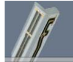
Figure 5-1 E-field Free-space Probe
