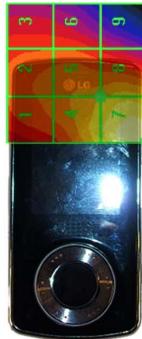
Figure 17-5 H-Field WD Scan overlay
