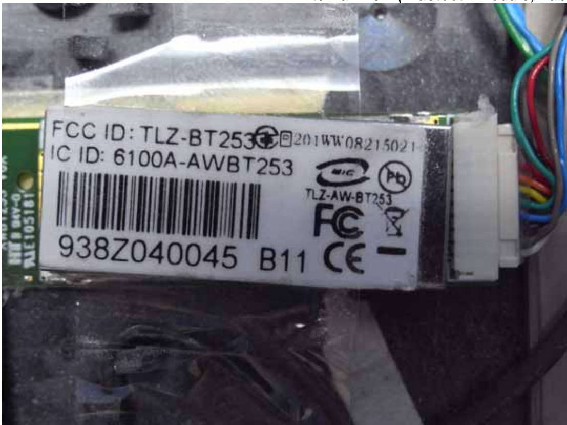
Figure 20 Internal View (Bluetooth Module, Label View)
