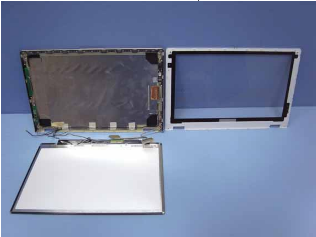
Figure 25 Internal View (Front Cover & LCD Panel Removed)
