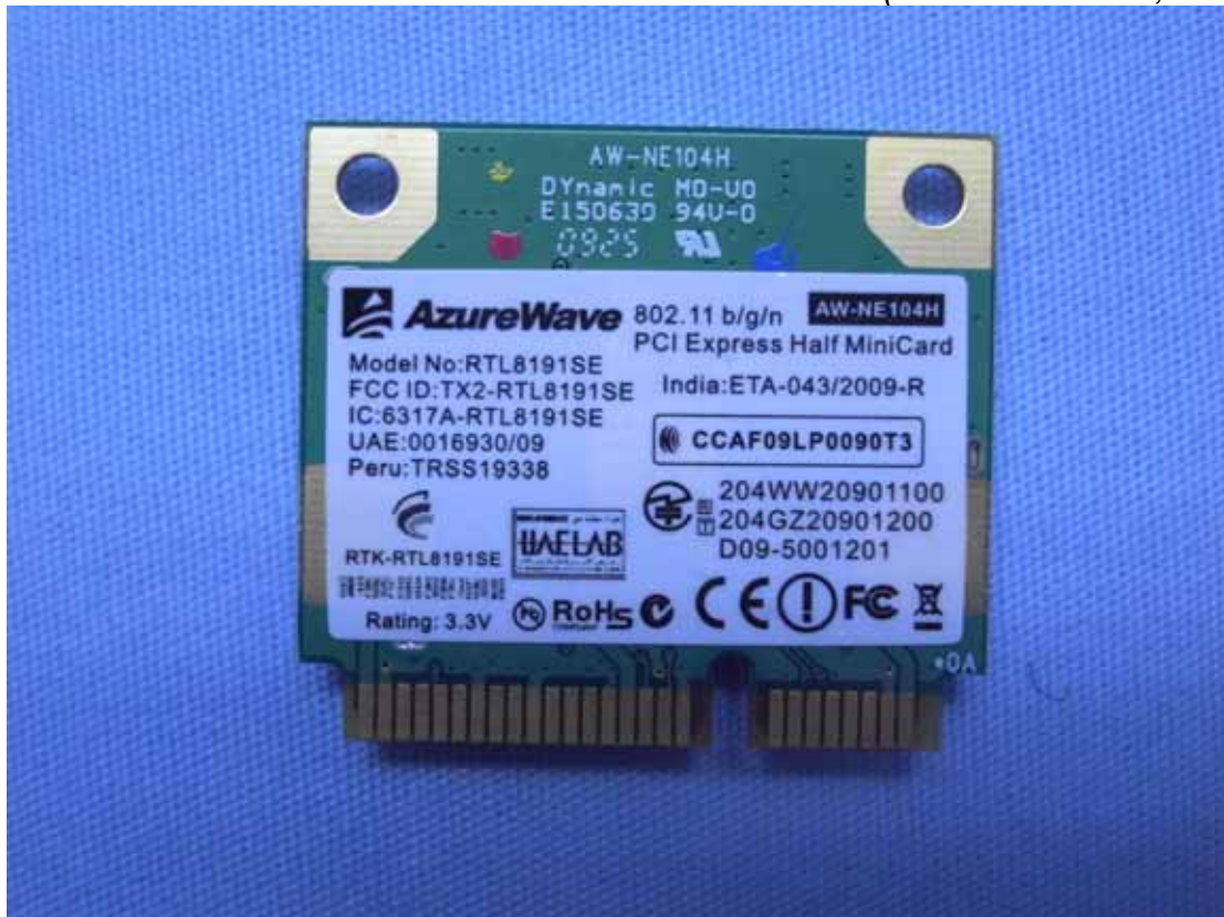
Figure 15 Internal View (Wireless Module, Back View)
