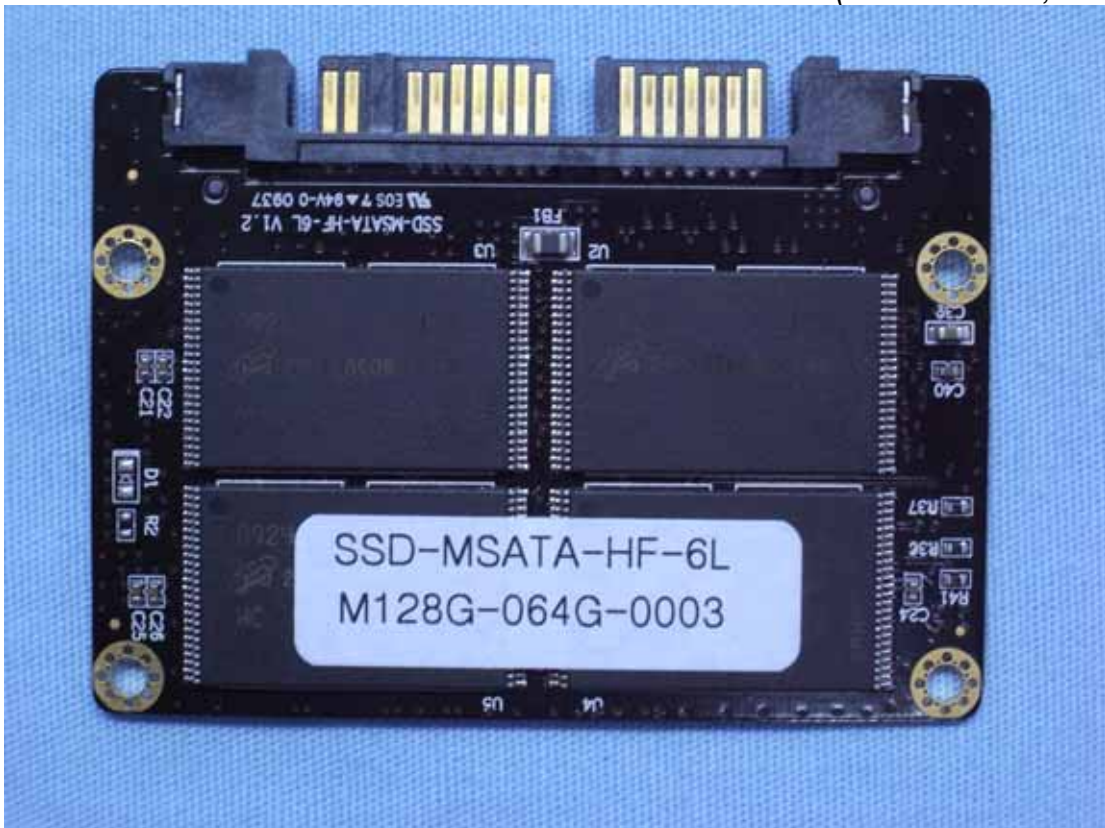
Figure 14 Internal View (Control Board, Back View)
