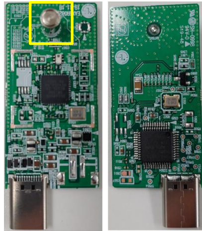
Picture. Module actual photo without Shield-Can (Left: TOP, Right: BOTTOM)
