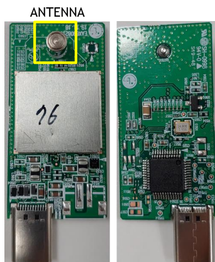
Picture. Module actual photo with Shield-Can (Left: TOP, Right: BOTTOM)
