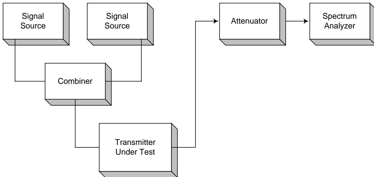
**Para. No. 2.991 - Spurious Emissions at Antenna Terminals**
