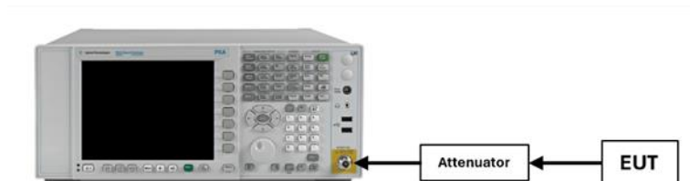
Figure 7-5. Test Instrument & Measurement Setup
