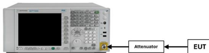
Figure 7-3. Test Instrument & Measurement Setup
