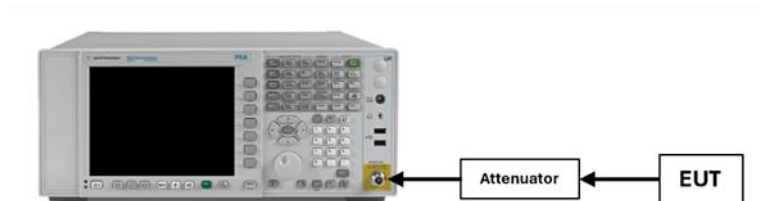
Figure 7-5. Test Instrument & Measurement Setup
