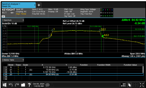
Figure 181 - 802.11ac VHT80 Maximum 99% OBW
