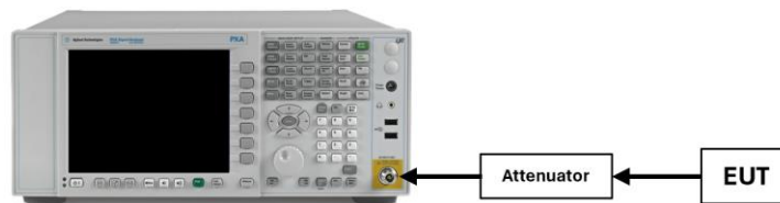
Figure 7-3. Test Instrument & Measurement Setup
