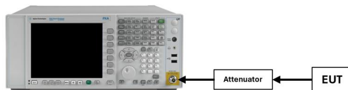
Figure 7-5. Test Instrument & Measurement Setup
