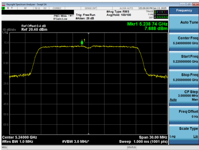
Plot 7-26. PSD Antenna 1b (20MHz BW 11ax– RU242 – Ch.48)
