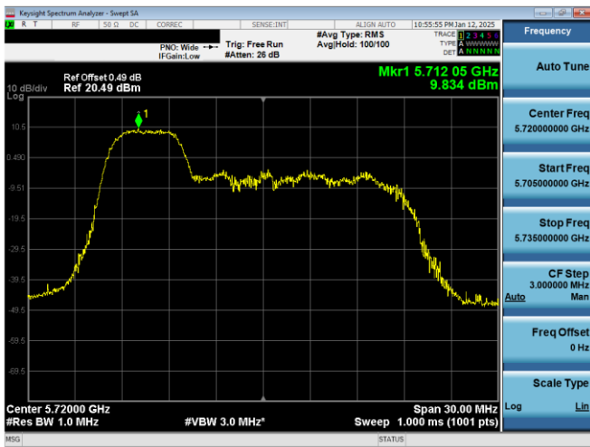
Plot 7-13. PSD Antenna 3c (20MHz BW 11ax Index 37 – RU52 – Ch.144)
