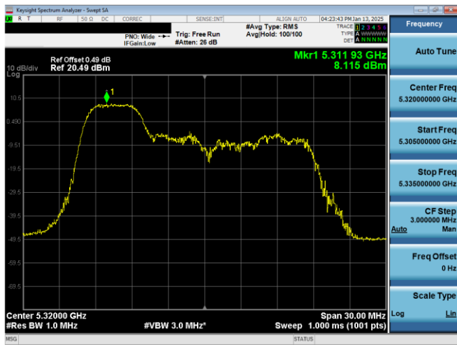
Plot 7-25. PSD Antenna 1b (20MHz BW 11ax Index 37 – RU52 – Ch.64)
