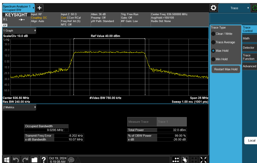
Plot 7-14. Occupied Bandwidth Plot (LTE Band 26/5 - 10MHz 16-QAM - Full RB Configuration)
