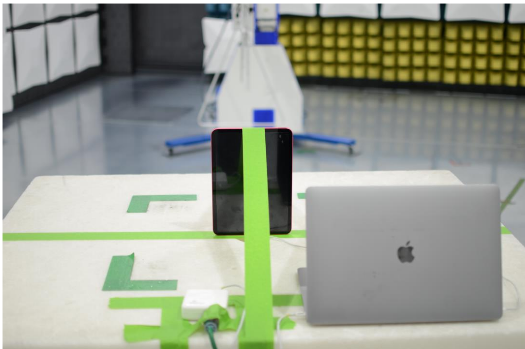
Figure 22: 30MHz-1GHz Test Setup (Rear View)
