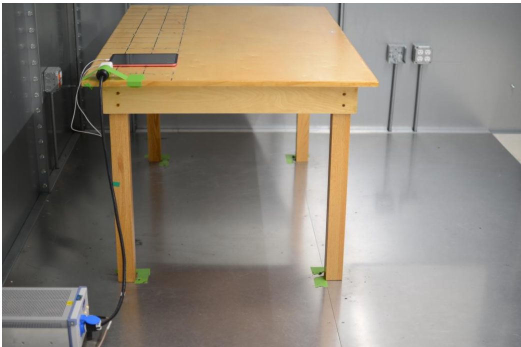
Figure 2: AC Line Conducted Emissions (Side View)
