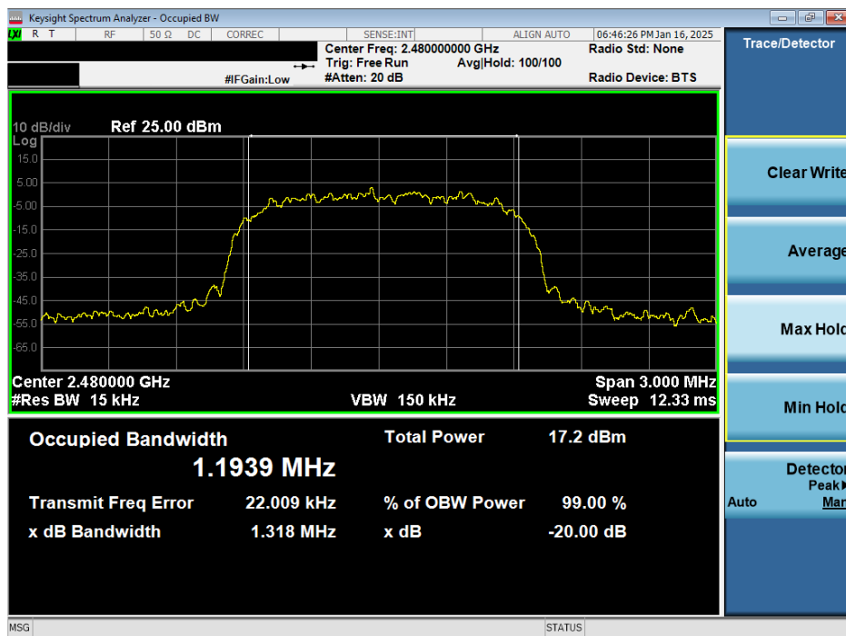
Plot 7-24. 20dB BW and 99% OBW Plot Antenna WF7b (Dedicated) (Bluetooth, 8DPSK, iPA – Ch. 78)
