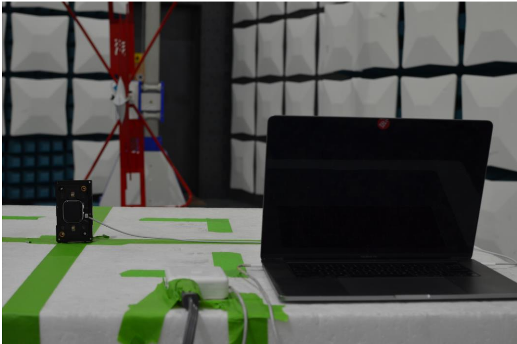
Figure 19: 30MHz-1GHz Test Setup (Rear View)
