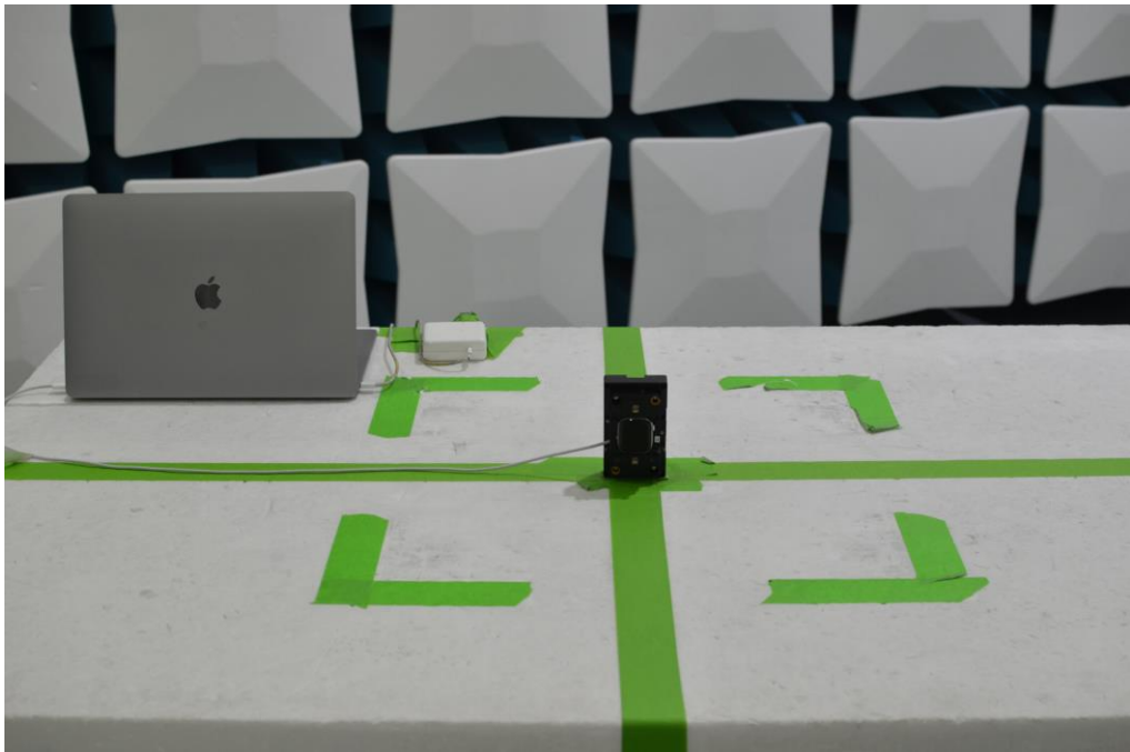
Figure 18: 30MHz-1GHz Test Setup (Front View)
