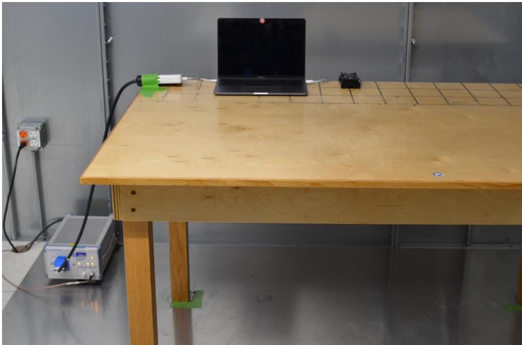
Figure 1: AC Line Conducted Emissions (Front View)
