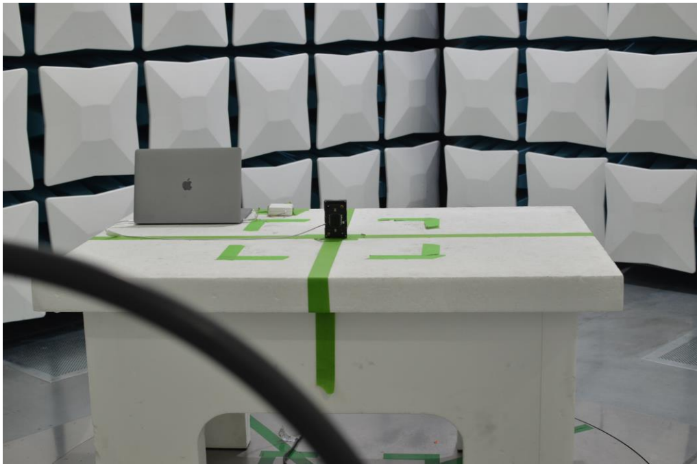
Figure 20: 9kHz-30MHz Test Setup (Front View)
