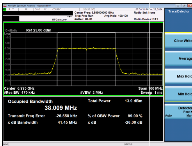
Plot 7-110. 26dB & 99% Bandwidth Plot Antenna 3b (40MHz 802.11ax RU484 (UNII Band 8) – Ch. 187)
