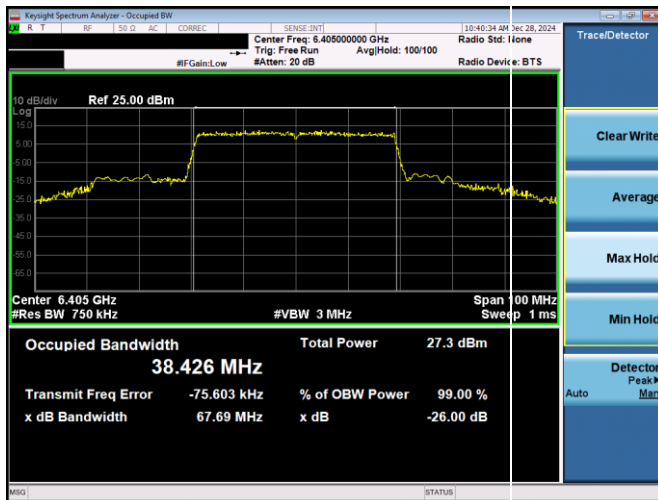
Plot 7-118. 26dB & 99% Bandwidth Plot Antenna 1b (40MHz 802.11ax RU484 (UNII Band 5) - Ch. 91)
