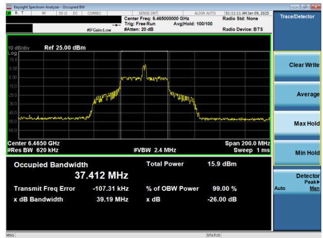
Plot 7-123. 26dB & 99% Bandwidth Plot Antenna 1b (80MHz 802.11ax RU26 (UNII Band 6) – Ch. 103)
