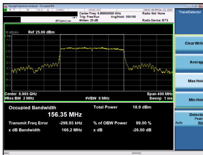
Plot 7-112. 26dB & 99% Bandwidth Plot Antenna 3b (160MHz 802.11ax RU26 (UNII Band 8) – Ch. 207)
