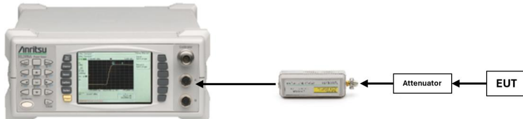
Figure 7-2. Test Instrument & Measurement Setup
