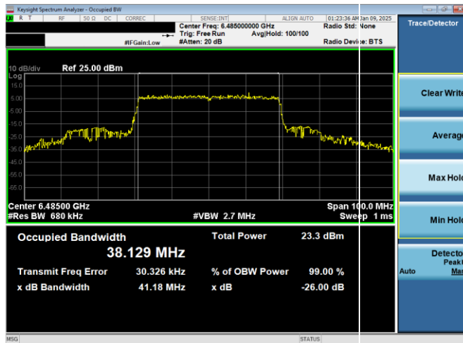
Plot 7-126. 26dB & 99% Bandwidth Plot Antenna 1b (40MHz 802.11ax RU484 (UNII Band 6) – Ch. 107)
