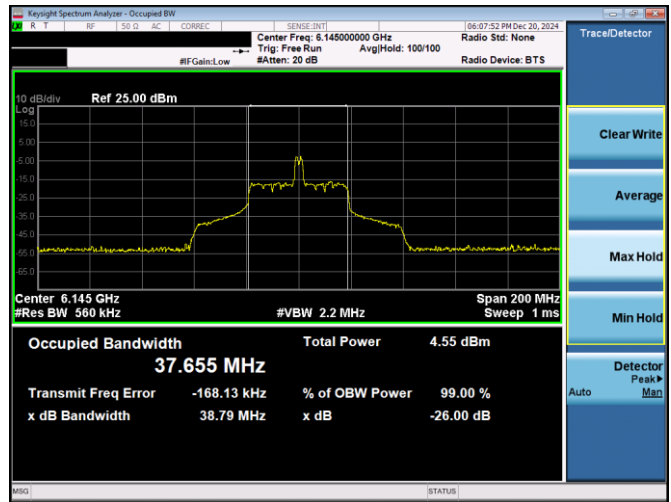
Plot 7-27. 26dB & 99% Bandwidth Plot Antenna 5T (80MHz 802.11ax RU26 (UNII Band 5) – Ch. 39)
