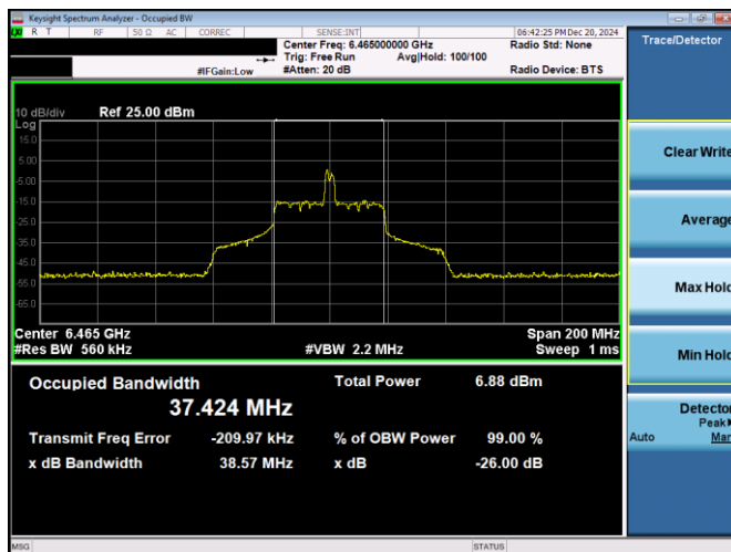
Plot 7-35. 26dB & 99% Bandwidth Plot Antenna 5T (80MHz 802.11ax RU26 (UNII Band 6) – Ch. 103)
