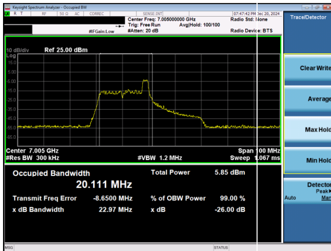
Plot 7-50. 26dB & 99% Bandwidth Plot Antenna 5T (40MHz 802.11ax RU26 (UNII Band 8) – Ch. 187)
