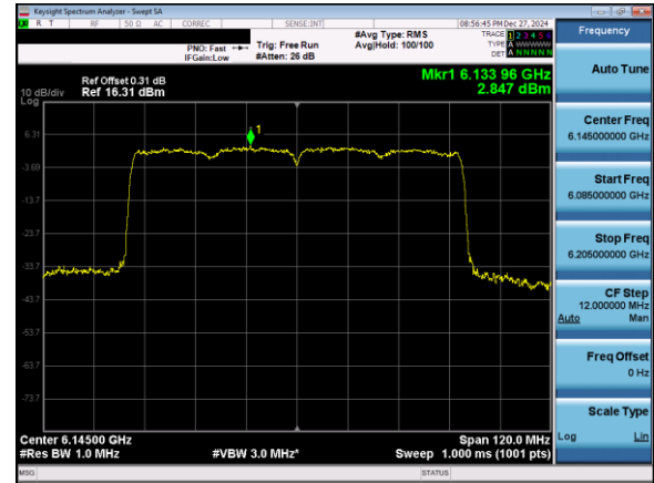
Plot 7-173. Power Spectral Density Plot CDD Primary Antenna 5T (80MHz 802.11ax (UNII Band 5) – Ch. 39)
