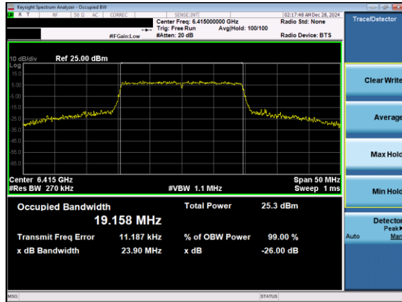
Plot 7-29. 26dB & 99% Bandwidth Plot Antenna 3b (20MHz 802.11ax (UNII Band 5) – Ch. 93)
