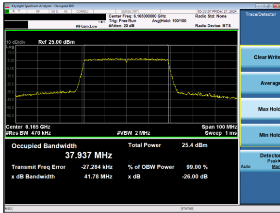
Plot 7-2. 26dB & 99% Bandwidth Plot Antenna 5T (40MHz 802.11ax (UNII Band 5) – Ch. 43)
