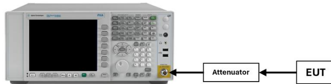
Figure 7-4. Test Instrument & Measurement Setup
