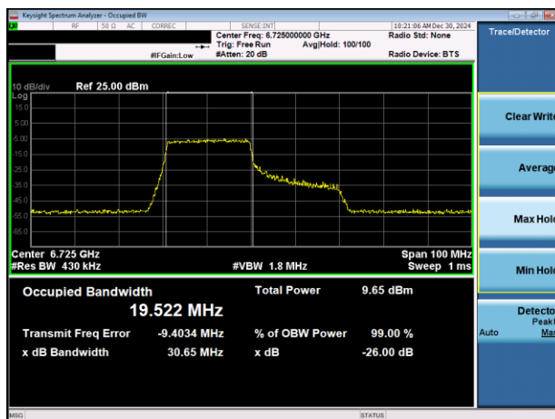
Plot 7-9. 26dB & 99% Bandwidth Plot Antenna 5T (40MHz 802.11ax RU242 (UNII Band 7) – Ch. 155)
