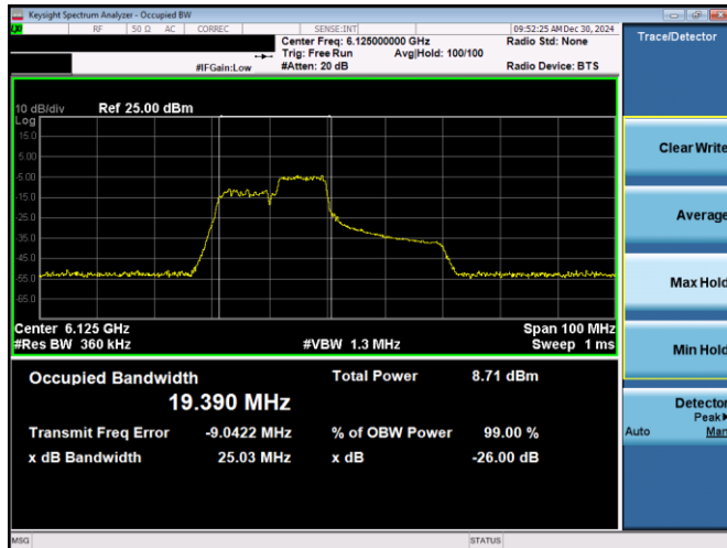
Plot 7-2. 26dB & 99% Bandwidth Plot Antenna 5T (40MHz 802.11ax RU106 (UNII Band 5) – Ch. 35)
