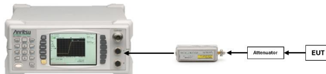
Figure 7-2. Test Instrument & Measurement Setup
