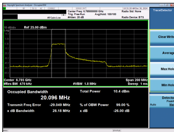
Plot 7-10. 26dB & 99% Bandwidth Plot Antenna 5T (80MHz 802.11ax RU242 (UNII Band 7) – Ch. 167)
