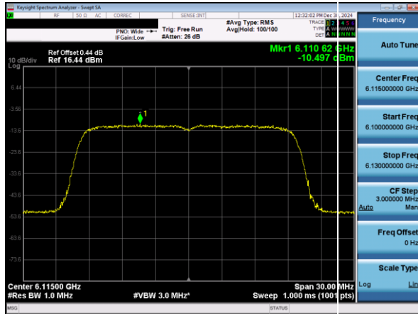
Plot 7-65. Power Spectral Density Plot SDM Diversity Antenna 5T (20MHz 802.11ax (UNII Band 5) – Ch. 33)
