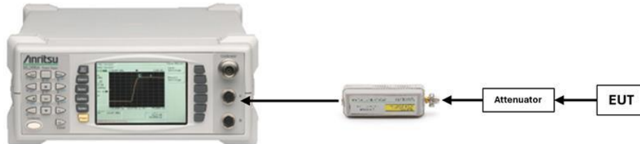
Figure 7-2. Test Instrument & Measurement Setup
